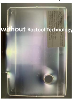
Result: The parts without Roctool technology (right picture) show more polarization and accordingly more internal stress. Especially at the weld line.
