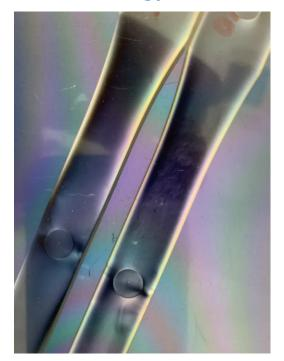
Results: On the tensile bars the difference of polarization and weld line visibility is not so distinctive.
