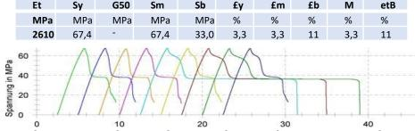
Results: Roctool Technology shows nearly similar mechanical properties than standard TOPAS tensile test. The tensile bars molded by Roctool without their molding technology shows brittle behavior.
