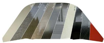
Photo: Materials tested on Large LIT (Light induction tooling) hood. The RocTool process enhances both cycle time and surface appearance on a multitude of thermoset and thermoplastic materials, and will be available to IACMI members starting mid-2017.
