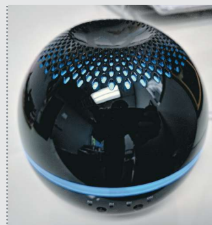
Flex molded this two-piece, snap-fit sphere of glass-filled PC with Roctool H&C technology, demonstrating the adaptability of flexible induction heaters to complex part shapes.
