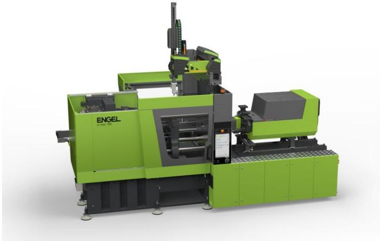
Featuring smart assistance, the all-electric e-mac injection moulding machine automatically compensates for fluctuations in the raw material to ensure consistently high part quality.
