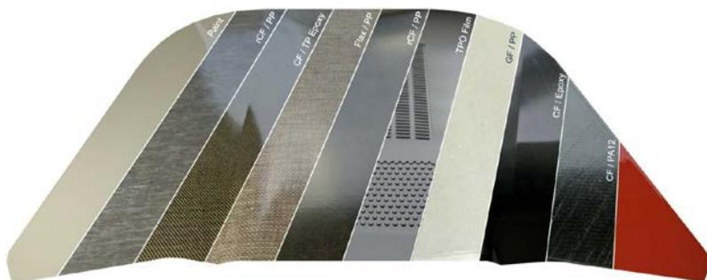
*Photo: Materials tested on Large LIT (Light induction tooling) hood. The RocTool process enhances both cycle time and surface appearance on a multitude of thermoset and thermoplastic materials, and will be available to IACMI members starting mid-2017.*
